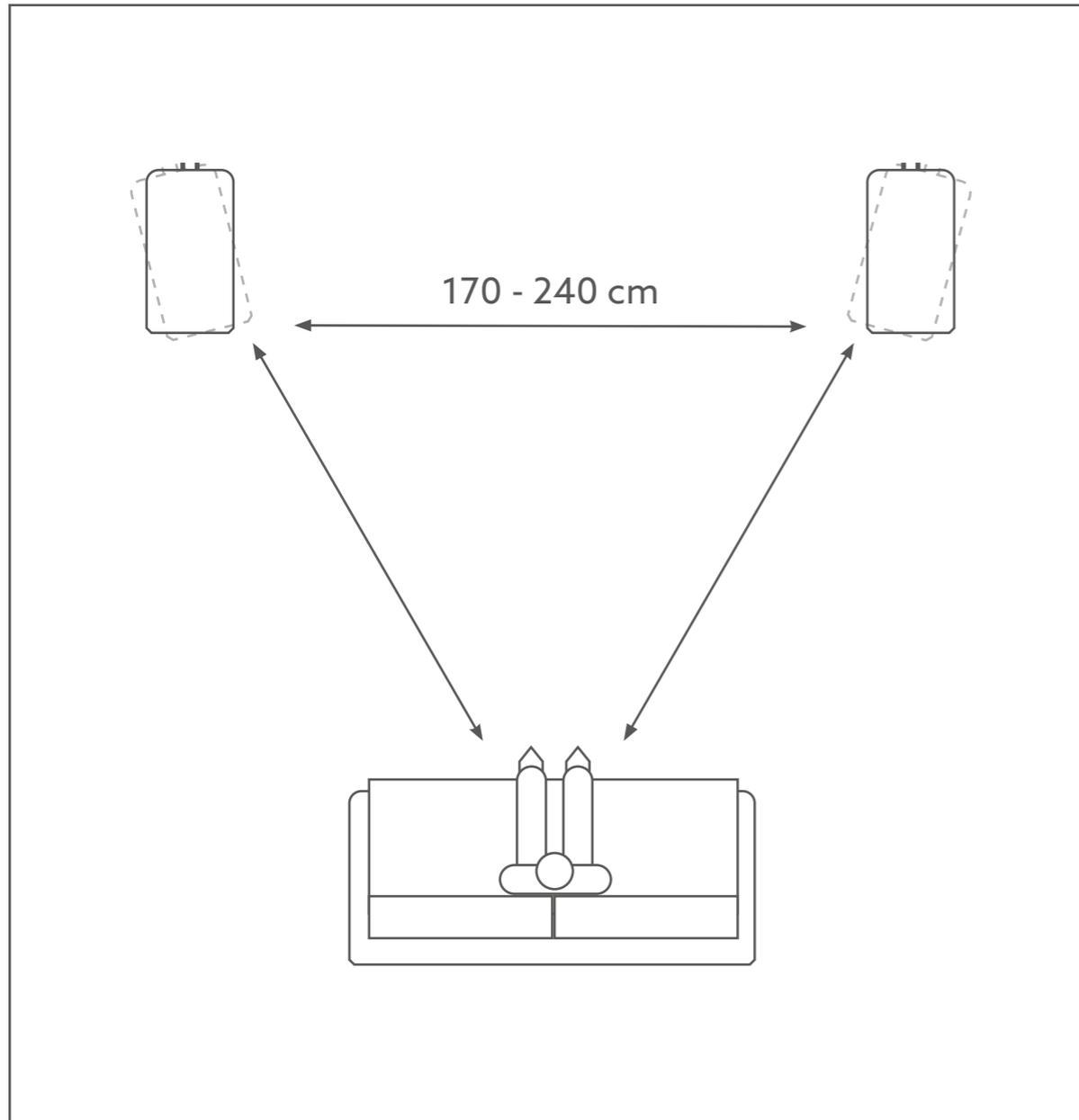
The position of the walls surrounding the loudspeaker has an impact on the sound of the loudspeaker. The more walls and surfaces there are in close proximity to the loudspeakers, the stronger the effect of the low and mid-range frequencies.
