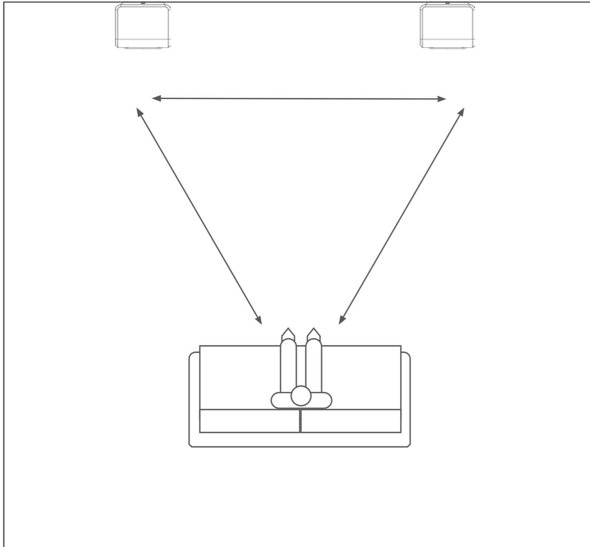
The position of the walls surrounding the loudspeaker affects the sound of the loudspeaker. The tuning of the AYERS Wall takes this into account exactly.
